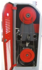
stabiler Riemenantrieb solid and smooth belt run
