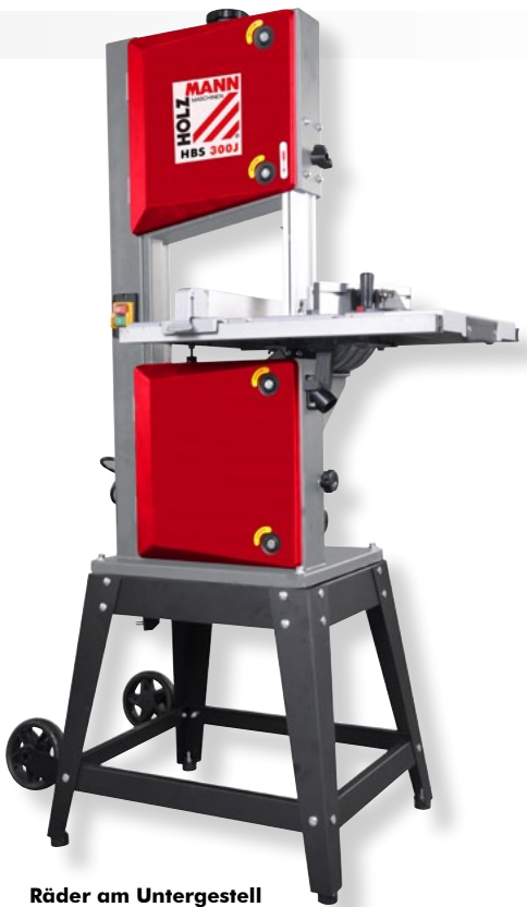
Räder am Untergestell wheels mounted on the stand
