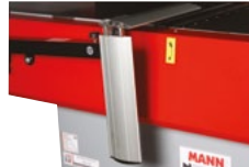
klappbare CPS Hobelwellenabdeckung CPS cutter block protection
